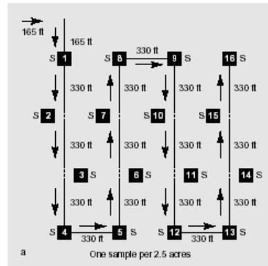
Directions for collecting soil samples from a 40 acre field. Each step is a 3 foot distance. Each numbered area is a soil sample location 20 ft. square. Five core samples 1 inch in diameter are collected from each square to a depth of 7 inches and mixed. (Fig 2)
