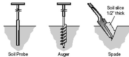
How to take soil samples with an auger, soil tube, and spade. (Fig 1)
